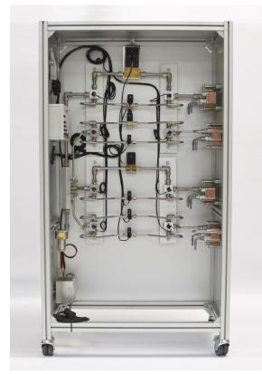
CRMT has designed and developped Gas Customizer to reproduce the composition of fossil natural gas, bio gas, hythane or any other alternative fuel gas, in order to test and adapt the engine in its actual conditions of use. The system allows for :
